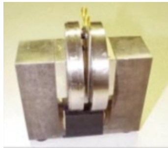
Figure 3.1: Image of Chuang and Gershenfeld’s tabletop Quantum Computer (from [23])
